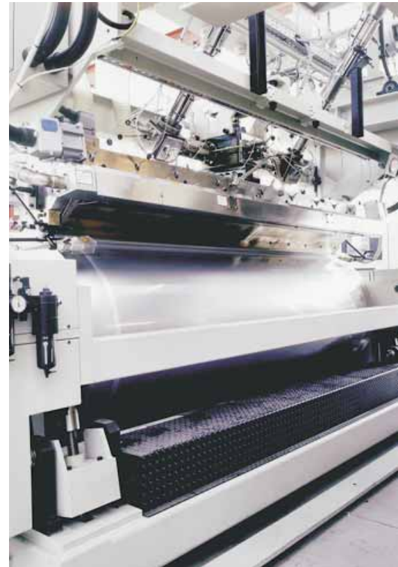
▲ The T-Die position over the Chill Roll is particularly studied for the perfect extrusion
