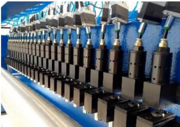
This device **OCCUPIES LITTLE SPACE** and is designed to punch **MACRO HOLES** of various diameters and shapes in **MOVING MATERIAL** and in particular, it works with **PLAIN OR PRINTED FILM**. This model has to be integrated into existing machinery such as extruders, slitters, bag machines etc. It is suitable to make holes on fruits and vegetables bags, garbage bags, paper bags, foam etc.
