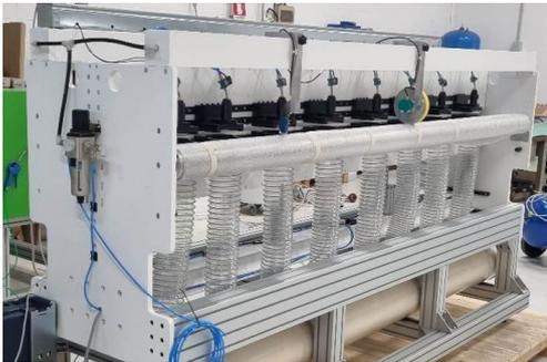
This is a **FAST AND STABLE DEVICE** designed to punch **MACRO HOLES** of various diameters and shapes in **MOVING MATERIAL** and in particular, it works with **PLAIN OR PRINTED FILM**. This model has to be integrated into existing machinery such as extruders, slitters, bag machines etc. It is suitable to make holes on fruits and vegetables bags, garbage bags, paper bags, foam etc.
